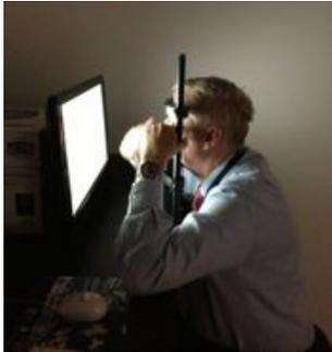
**Figure 7. 3D-CTAG test setup at NSBRI on height-adjustable table in a room with controlled lighting (top). Test subject on chin-head rest in front of touchscreen at a fixed distance performing the visual field test (left).**
