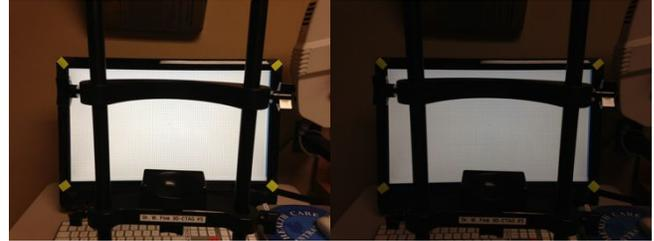
**Figure 6. Left: Eccentric fixation markers in yellow before the testing (i.e., lights on). Right: Fixation markers fluoresce after the test procedure has begun (i.e., lights out).**
