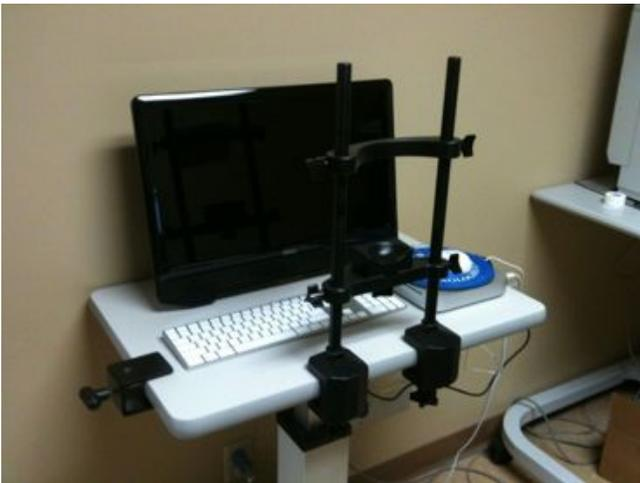
**Figure 3. Examination station setup for 3D-CTAG consisting of an Apple Mac mini computer, a head-chin rest, and a touch-sensitive computer monitor.**
